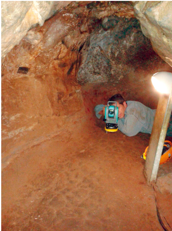
Figure 6 Surveying the lower underground passages of the Sterkfontein Caves. Here S. Brown is surveying datum 11 from datum 10 of Underground Traverse B (FIGS 4 and 5). This is part of the tourist route through the caves. Traverse C established datums away from the tourist accessible areas.
